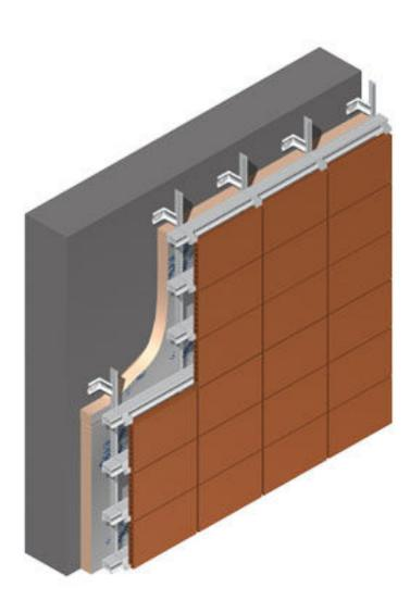
Kingspan Kooltherm K15 Rainscreen Board is the first insulation board to achieve LABC approval.
